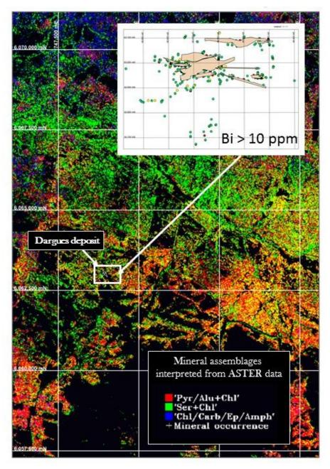
Figure 2. Interpreted ASTER mineral map with the location of the Dargues deposit. Inset shows the distribution of Bismuth (Bi) around the Dargues Resource. All Bi > 10 ppm shown. Hatched orange shapes are the Resource wireframes in plan view. Grid is MGA94 and grid spacing is 2500m in the main frame and 100m in the inset.
